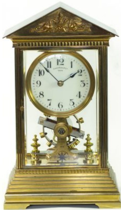
Architectural Eureka clock, electromagnetic movement with large balance wheel , dated c.1910
