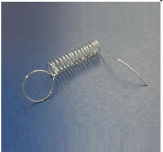
These silver contact springs are fitted to the Bulle with one end attached to the end of the fork arbour and the other by a small rotatable brass tag. The fork has a small silver grove in which the spring, with it's large loop end, rolls on each side to side movement of the pendulum. It serves three purposes.
