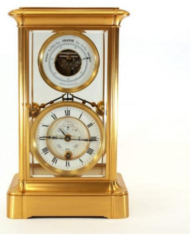
An exceptionally rare year-going four-glass clock. The timepiece movement has a single going barrel providing power to a Leroux-type deadbeat escapement. This in turn drives the equipoise compound pendulum beating seconds. The very fine pallets are fixed rigidly to the pendulum and the impulse is provided by the profile of the escape-wheel teeth.
